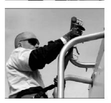
Hold the TRAM handhold with both hands and depress the clutch lever to allow the TRAM arm to rise.
