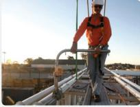
The proven TRAM Fall Protection System, with thousands of units installed worldwide, is now available for cranes and derricks. The TRAM system provides fall restraint or arrest protection as well as an integrated, adjustable handhold for both stability and confidence. TRAM is the only system available that combines all of the following:
