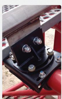
The proven TRAM Fall Protection System, with thousands of units installed worldwide, is now available for Lattice Boom Crawler cranes. The TRAM system provides fall restraint or arrest protection as well as an integrated, adjustable handhold for both stability and confidence.
