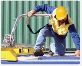
**ISO TRAM** Fall Protection System is specifically designed to protect those working on ISO containers. The system consists of a rail-mounted TRAM unit fixed to a transportable frame. The frame is lifted into place by a light forklift and then locked into position at the ISO connections. It can be supplied with or without a ladder and walkway.
