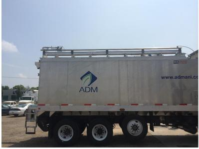
The proven TRAM Fall Protection System, with thousands of units installed worldwide, is now available for Agricultural Feeders. The TRAM system provides fall restraint or arrested protection as well as an integrated, adjustable handhold for both stability and confidence.
