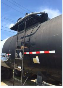
The proven TRAM Fall Protection System, with thousands of units installed worldwide, is now available for Dome Tankers. The TRAM system provides fall restraint or arrested protection as well as an integrated, adjustable handhold for both stability and confidence.
