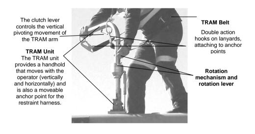
The TRAM and horizontal rail has been tested to the specifications of, and is compliant with:
