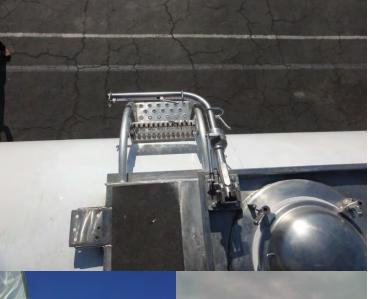
The proven TRAM Fall Protection System, with thousands of units installed worldwide, is now available for General Transportation. The TRAM system provides fall restraint or arrested protection as well as an integrated, adjustable handhold for both stability and confidence.
