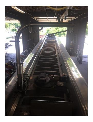
The proven TRAM Fall Protection System, with thousands of units installed worldwide, is now available for Transformer Oil Trucks. The TRAM system provides fall restraint or arrested protection as well as an integrated, adjustable handhold for both stability and confidence.
