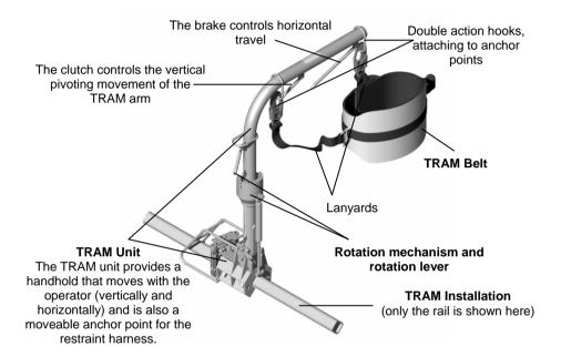
The TRAM and horizontal rail has been tested to the specifications of, and is compliant with:
