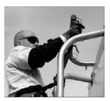
Hold the TRAM handhold with both hands and depress the clutch lever to allow the TRAM arm to rise.
