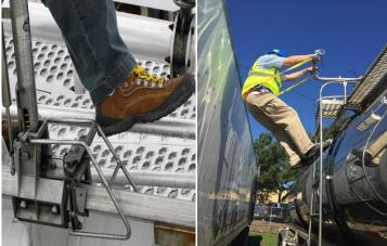
The proven TRAM Fall Protection System, with thousands of units installed worldwide, is now available for Side Ladder Access Trucks. The TRAM system provides fall restraint or arrested protection as well as an integrated, adjustable handhold for both stability and confidence.
