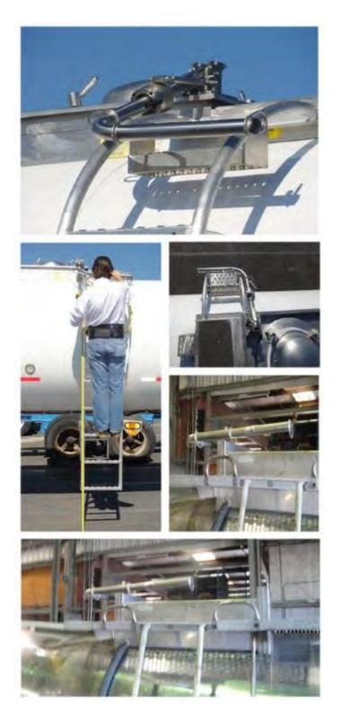
The proven TRAM Fall Protection System with thousands of units installed worldwide isnow available for Single Dome Tankers. The TRAM system provides fall restraint or arrested protection as well as an integrated & adjustable handhold for both stability and confidence.
