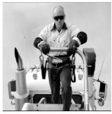
Disconnect lanyard hooks from the TRAM and reattach to the belt in the 'carry position'
