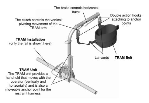
The TRAM and horizontal rail has been tested to the specifications of, and is compliant with:
