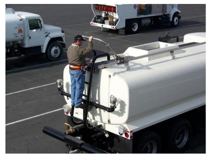
The proven TRAM Fall Protection System, with thousands of units installed worldwide, is now available for Water Trucks. The TRAM system provides fall restraint or arrested protection as well as an integrated, adjustable handhold for both stability and confidence.
